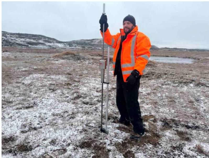
Photograph 18 Dynamic Cone Penetration Test – Point 10
