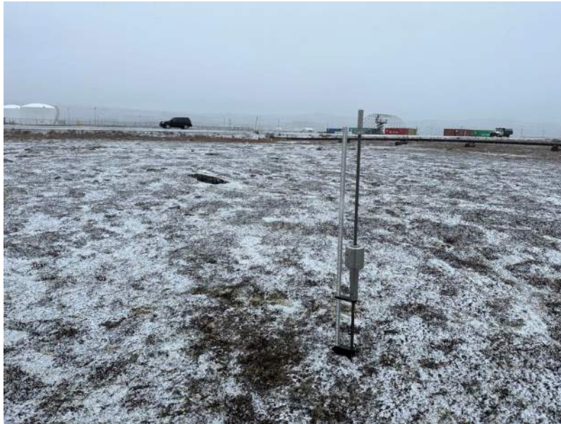
Photograph 17 Dynamic Cone Penetration Test – Point 2
